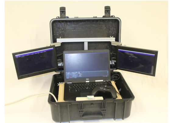
Topside control box
